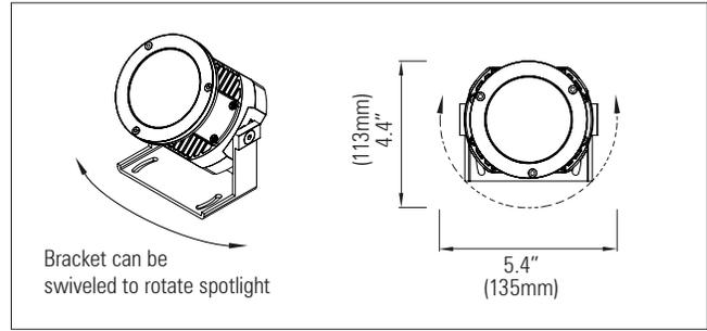
**D 100 IP20 Spotlight with 1 x high-power tunable white LED cluster array comprising of 4 x white-light LEDs, with ultra narrow beam collimator lens**
